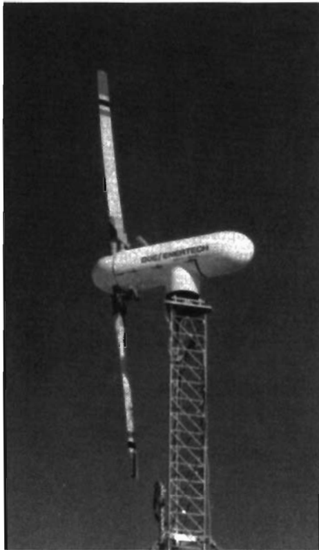
(a) Horizontal-axis wind turbine
